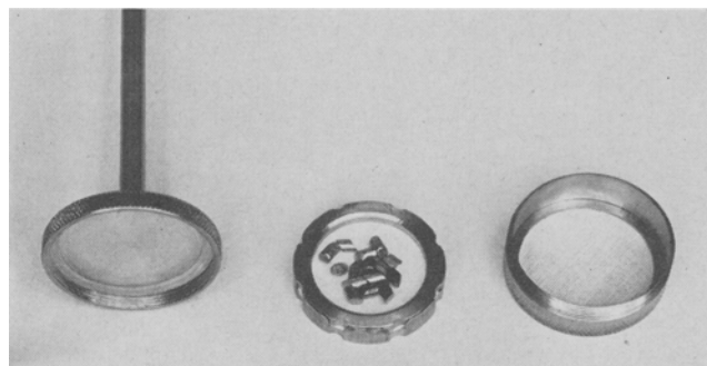
FIG. 6. Miniature wash vessel of type 2 washer disassembled, showing soiled cloth discs in ring assembly and redeposition disc in bottom portion.
