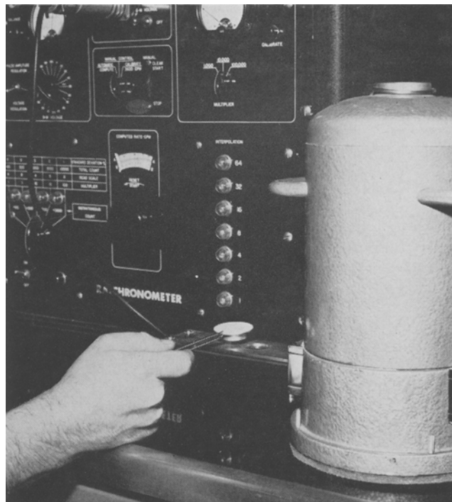
Fig. 3. Arrangement for measuring radioactivity of soiled cloth discs.
